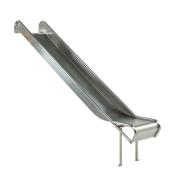
Stainless steel slide - The high quality of the materials used and solid welding guarantees high resistance to mechanical damage - 2 mm thick sheet metal, steel pipe fi 33,7 mm, durable linear welding.
