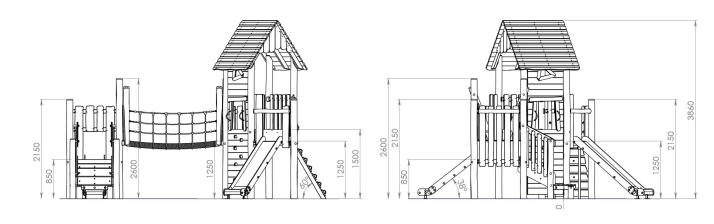
The playground equipment consists of two main parts with a thick rope bridge between them. It features two slides at different heights. The designed offer lower tower designed for toddlers to climb the stairs and slide. The 40 cm height to the right prevents smaller children to continue their movement onto the suspended bridge but facilitates the older to do that. The bigger structure consist of three platforms on two different levels and an inclined ramp.
