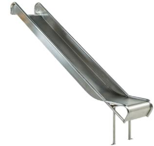
Stainless steel slide - The high quality of the materials used and solid welding guarantees high resistance to mechanical damage - 2 mm thick sheet metal, steel pipe fi 33,7 mm, durable linear welding.
